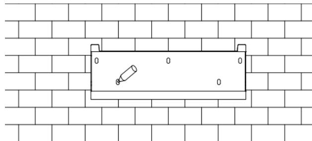
Drill holes with electric drill, make sure the holes are at least 50mm deep, and then tighten the expansion tubes.
